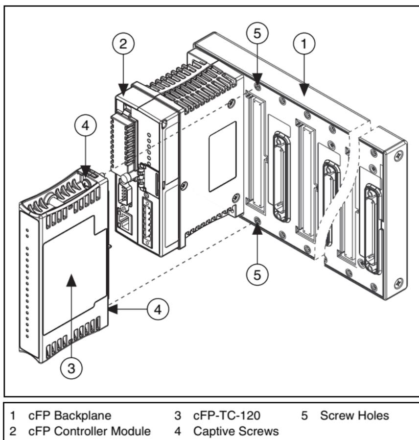
**Figure 2.** Installing the cFP-TC-120
