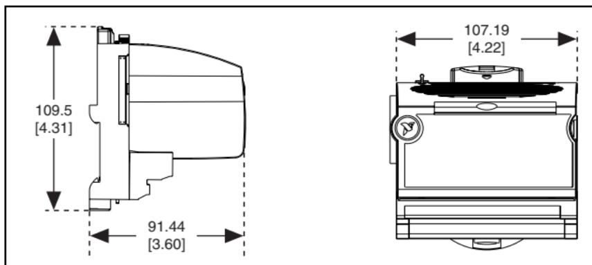
**Figure 10.** FP-TC-120 Mechanical Dimensions
