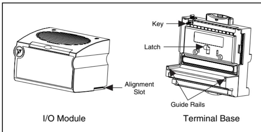
**Figure 1.** Installing the FP-TC-120
