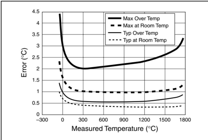
Figure 6. Type R and S Errors
